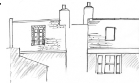
Number 9: a small leaded rear dormer with its french windows opening onto small hidden balcony space; and front conservation style rooflight on same centreline as bay below.
